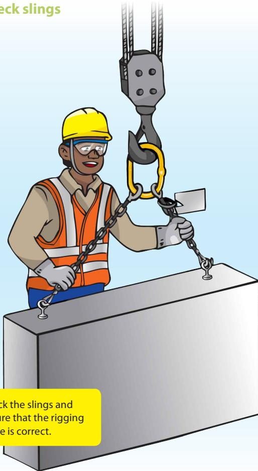
Check the slings and ensure that the rigging angle is correct.
