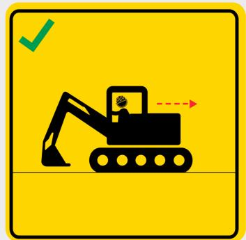
Switch off the excavator and remove the key before leaving cabin.
