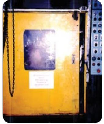
Figure 33: Sliding door was not fitted with an interlocking guard.
