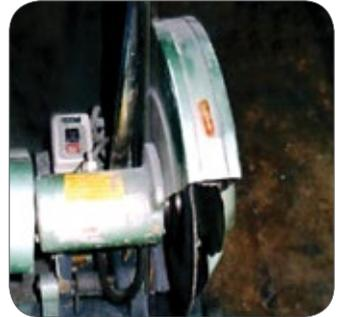
Figure 35: Rotating abrasive disc cutter.
