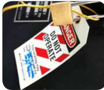
Figure 8: Machine locked-out and tagged-out for maintenance.
