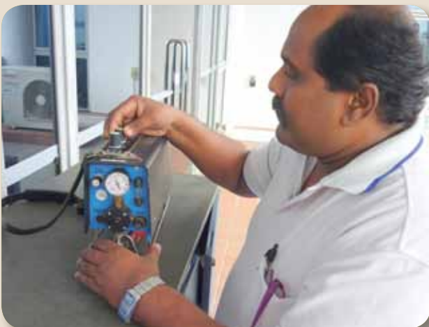
V Sandourajan Pandian (Technician from Gas Leak Vehicle Patrol Team, SP PowerGrid) checking the flame ionisation detector to ensure it is in working condition before setting off for patrol duties.
